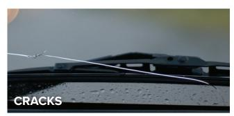
Curved or straight lines that extend across the windshield. They can also exist in one side of the windshield.
