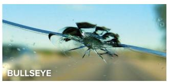
Usually circular windshield cracks and fractures that look similar to a target of concentric cracks.
