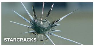
Extend from a central point of damage with long cracks.
